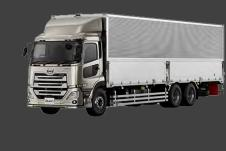
capacity volume has increased by shortening the cab length by 295 mm. The length of the loading platform has been extended to 10.02 meters, allowing extra room for cargo equivalent of two additional T11 pallets, compared to the full cab model.
